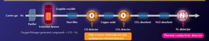
Oxygen determination : 2 NDIR detectors for high accuracy among the full measurement range. Automatically controlled by the software.
