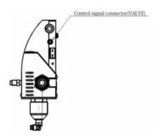
5) Fit the supplied thermocouple (MAIN TC) cable for mixing valve to the thermocouple (MAIN TC) connector on the mixing valve, and connect the thermocouple (VAPO TC) cable for vaporizer to the thermocouple (VAPO TC) connector on the vaporizer. Connect the heater cable (MAIN HT) for mixing valve to the heater connector (MAIN HT) on the mixing valve, and connect the heater (VAPO HT) connector for vaporizer to the heater (VAPO HT) connector on the vaporizer.
