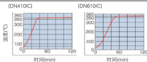
N<sub>2</sub>置换性能曲线
